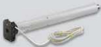
220V or 24V tubular motor, torque from 30Nm to 100Nm, IP44
